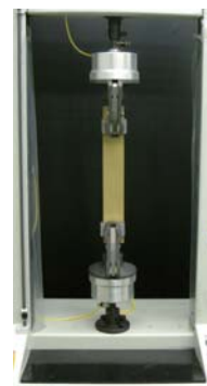
Tensile strength test method in accordance with JIS 1096-1990
