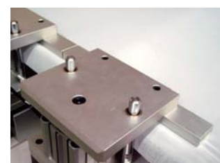
Automatic clamps grip mesh
