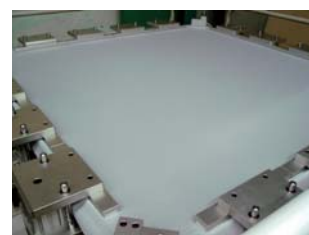
Fabric stretched to preset tension
